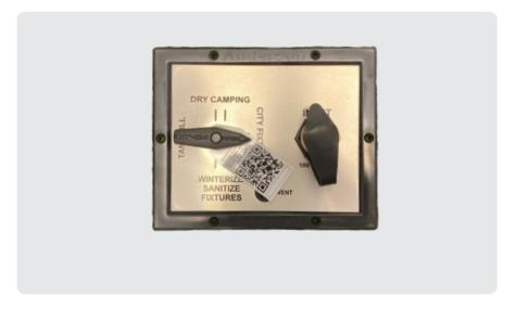
The MANRV101 RV Water Service Panel features an inlet 4 function (4 position) low lead brass valve that is used for filling the holding tank, pressurizing the fixtures when you have a water supply, pump from the tank during dry camping and help you with winterizing and sanitizing your unit.
