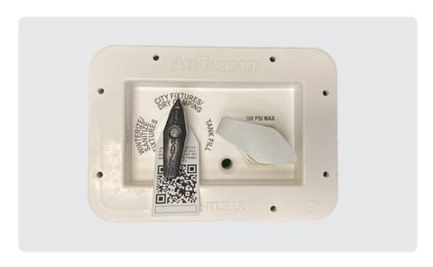
The MANRV101-RF RV Water Service Panel features an inlet 4 function (3 position) low lead brass valve that is used for filling the holding tank, pressurizing the fixtures when you have a water supply, pump from the tank during dry camping and help you with winterizing and sanitizing your unit.
